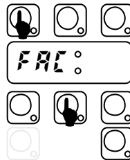
Fig. 1.5 Enter into Factory Parameters (Hold down buttons for at least five seconds).
